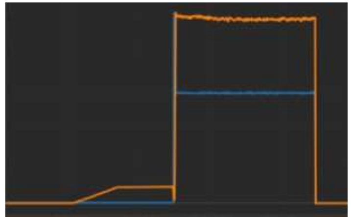
Thruster parameters during ignition in space (voltage and current) which confirm the nominal behaviour of the testing (Credits: Exotrail)
